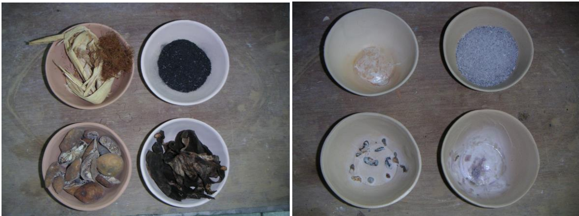
Fig. 4. Raw material after firing in the temperature 1200°C
