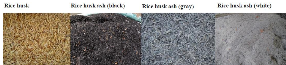
Fig. 2. Rice husk and 3 types of Rice husk ash.
