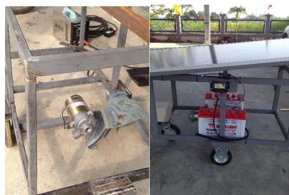
Fig.11 The installation of water pump and solar system
