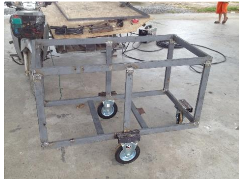
Fig.10 The structure of stroller of mobile solar water pump
