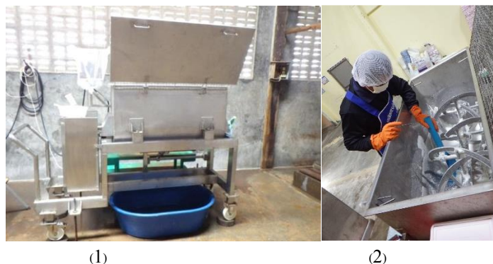
Figure 1 The iodine mixing machine(1) Large scale iodine mixing machine and (2) Inside the mixing chamber.
